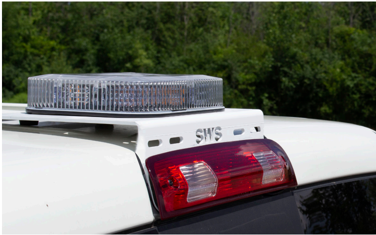
Low profile Third brake light platform Illustration: 98088FWH and Compact Select Minibar 10103P
